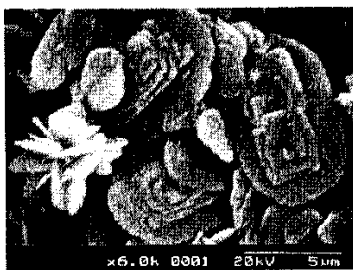
Fig. 2 Tabular crystals with pyramidal growth and rose aggregates obtained at lower supersaturation ratio ( S=10^3 ). Mode A, 25 mm; Q=150-15 \text{ l h}^{-1} ; N=600 \text{ rpm} . d_{43}=5.1 \mu\text{m}
