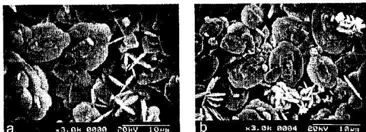
Fig. 3 Effect of the rotation speed on morphology: tabular crystals with pyramidal growth prevail, but smaller twin crystals form at lower speed (left photo) and rose aggregates form at higher speed (right photo). Feed mode B ( a=3 \text{ mm} ); S=10^4 ; Q=385 \text{ l h}^{-1} . a) N=200 \text{ rpm} , d_{43}=6.6 \mu\text{m} . b) N=900 \text{ rpm} , d_{43}=6.1 \mu\text{m}
